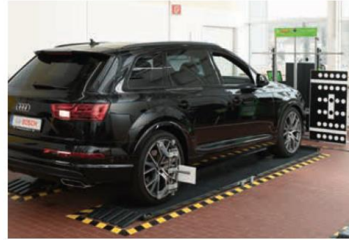
Audi: Double-Radar calibration with short setup time. Attach VW-Target to match with left and right radar axis. Lateral adjustment with a sense of proportion. Thanks to innovative product design, no height adjustment required.
