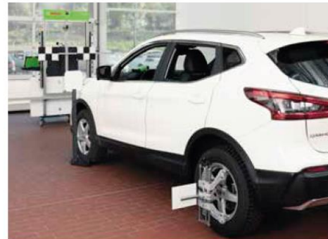
Nissan front radar + camera: The software based distance measurement shows it's full advantage especially at distances of 2-4 meter. That's a gain of workshop efficiency. Distance measurement aid with pointer for wheel centre reference.
