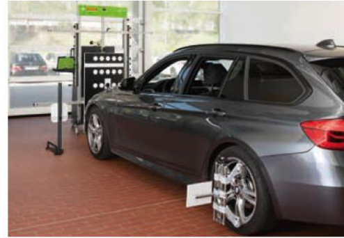
BMW/Mini and VW-Group: Highly precise placement towards the driving axis including specific distance setting. VW-Target installed vertical and centred in front of Radar sensor.
