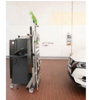
3-point radar calibration: Tilting positions according to OEM requirements: +2°, 0°, -2°
