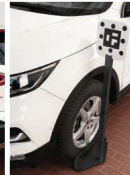
Nissan front radar + camera: The software based distance measurement shows it's full advantage especially at distances of 2-4 meter. That's a gain of workshop efficiency. Distance measurement aid with pointer for wheel centre reference.
