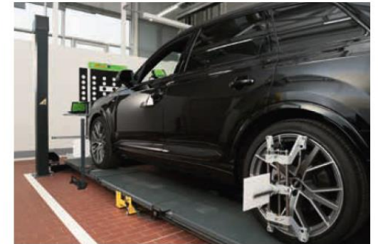
Above floor lifts: Program routine for permanent yaw angle display for monitoring if target is perpendicular to driving axis.
