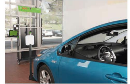
Toyota front camera: Sequential calibration with one or multiple targets. Highly precise positioning of the distance measurement aid according to OEM requirements.
