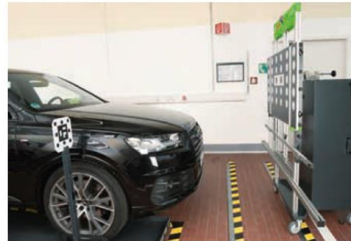
Headlight aimer bay: trouble-free placement between the rail systems. Ensured by large wheels, distance measurement aid and roll/pitch angel setting directly on the measurement bar.
